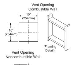
Figure 22 - Vent Opening Requirements
